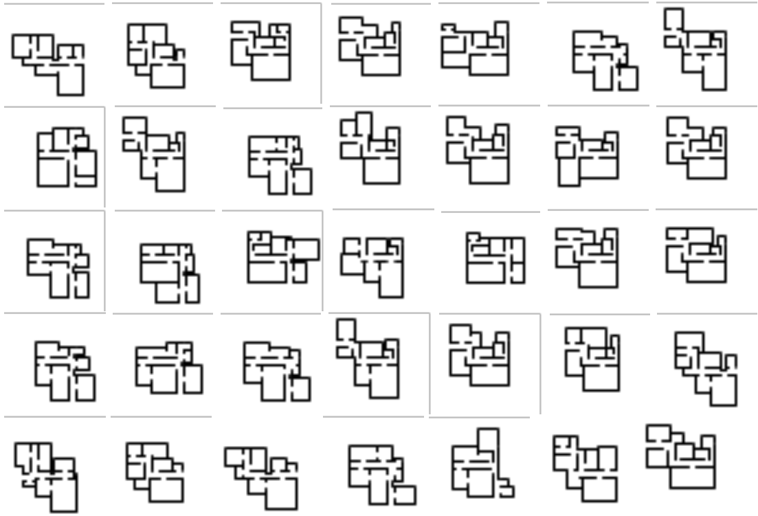
Figure 2: Examples of the final floor plan dataset, which consists of a 1000 binary images of two-bedroom apartments that possess passages between rooms and an entrance.
