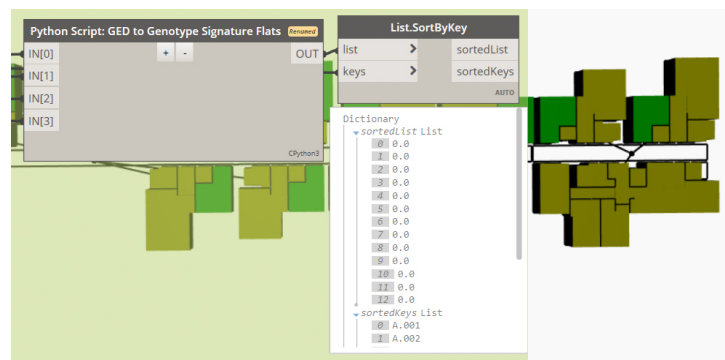
Figure 7: Genotype signature apartment layouts identified by the Evaluator script in a Revit test file, and rooms coloured based on the Ideal Room Sizes database.
