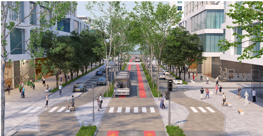
Figure 10: A rendering of the re-imagined Tzahal Street, combining high Place function with medium movement function and BRT infrastructure.
