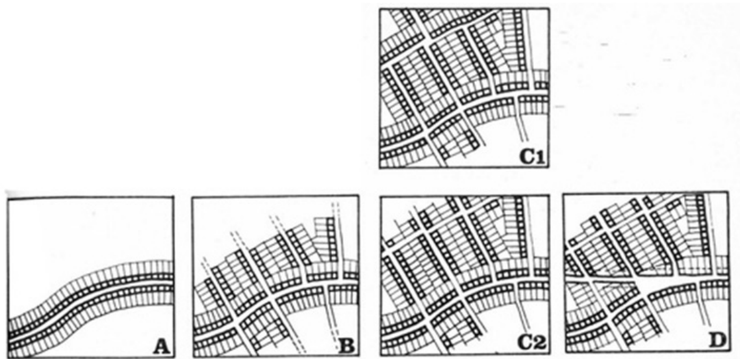
Figure 2: Successive processes of road network and built-up tissue formation according to Caniggia and Maffei (1979, 132): Arterial roads (A), access roads (B), connecting roads (C) and restructuring roads (D)
