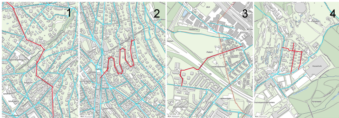
Figure 5: Examples of named routes deviating from continuous trajectories for different reasons. Bergstrasse (1) avoids slopes by following a contour line. Rigistrasse (2) climbs a steep slope in serpentine. Frohbühlstrasse (3) follows a contrived trajectory forced by the location of a highway underpass. Im Klösterli (4) covers all branches of the internal circulation system of a residential neighbourhood constructed in 1937. Background map source: www.maps.stadt-zuerich.ch
