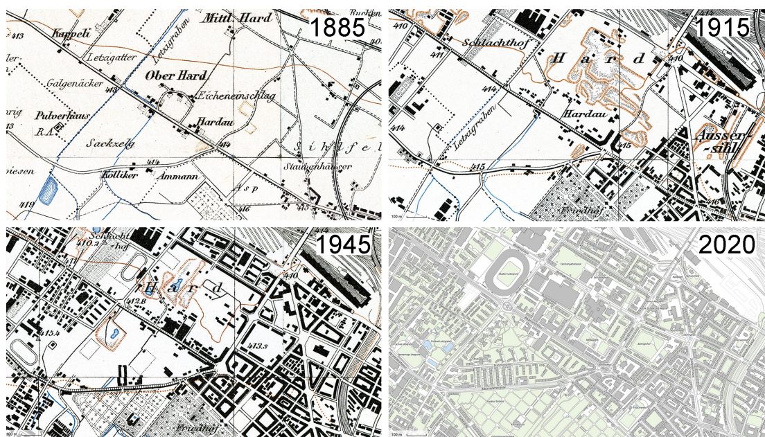
Figure 6: Temporal evolution of the route network in the Hardau area west of the city centre in 1885 (top left), 1915 (top right), 1945 (bottom left) and 2020 (bottom right). Map source: www.maps.stadt-zuerich.ch .
